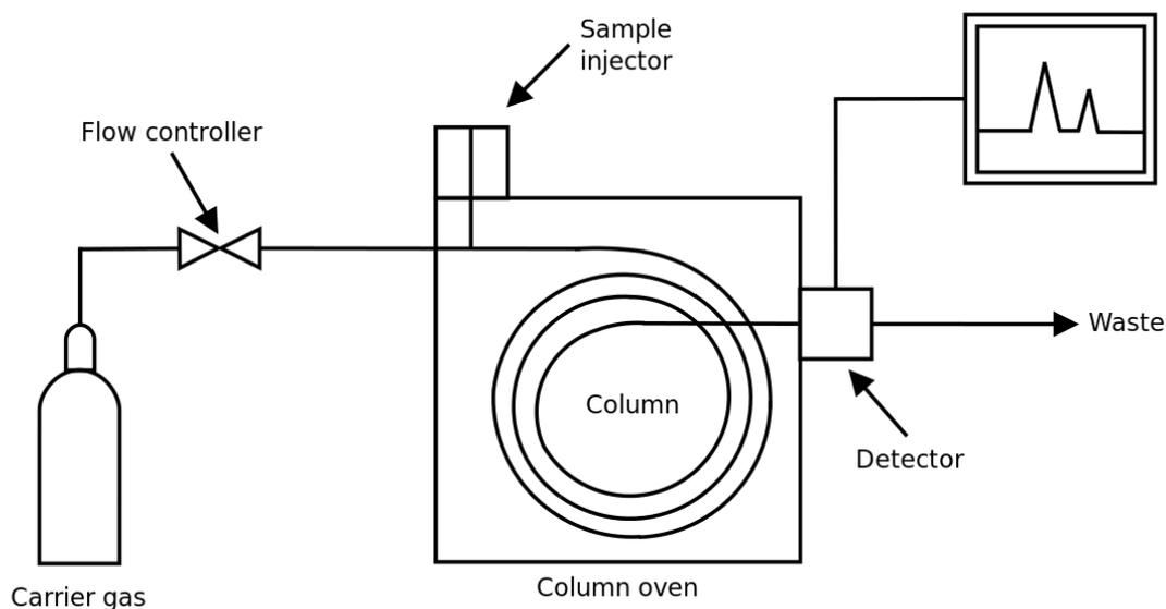
**Figure 6:** Basic overview of a gas chromatograph (GC). As the carrier gas enters the system through the flow controller, it carries the sample through the column. There, the components of the compound are separated by their characteristics such as size and ability to adhere to the column coating. (Figure citation: Gas chromatography, 2016).
